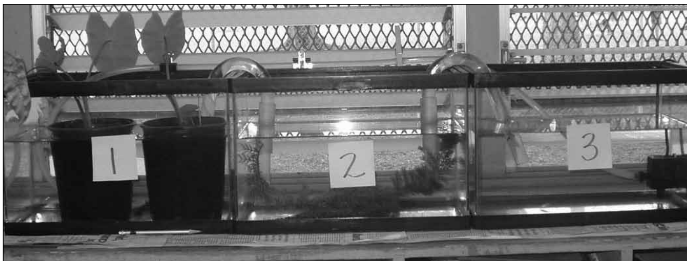
Fig. 1. Example of a system designed by teachers that housed a natural ecosystem and treated aquarium wastewater. Tank 3 contains fish, the waste producer. Tanks 2 and 1 contain aquatic plants and substrates (rocks) for microorganisms.
